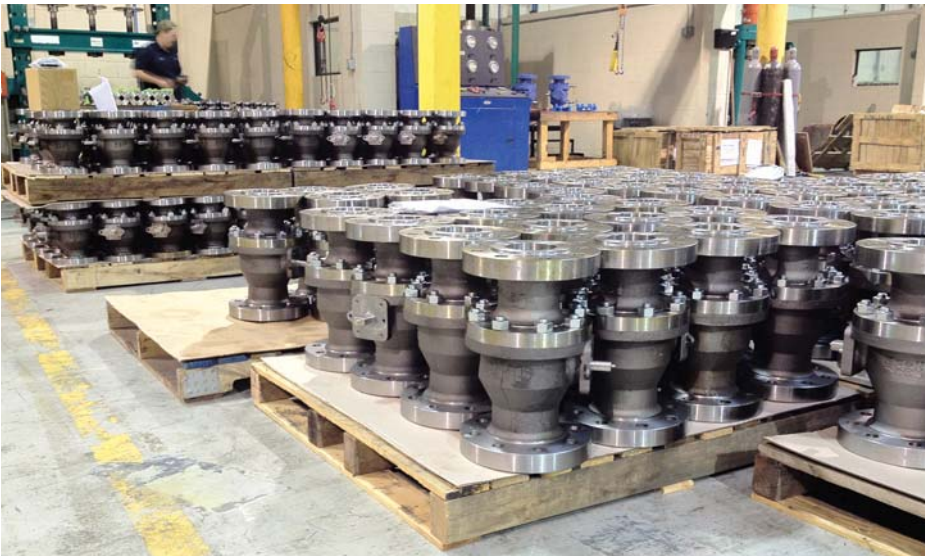
ViNtrol Valves staged for Hydro Test.
